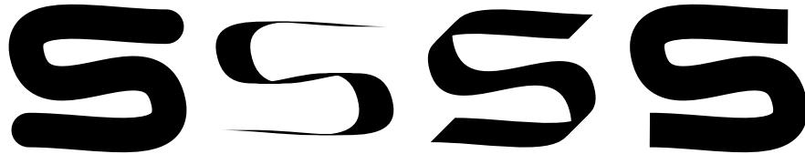
The same path is drawn in four different ways: First, using a thick, but otherwise ordinary, pen. For the next two images we have used a flat pen in two different orientations. (Note that the global **penscale** declaration applies only to the default pen.)
