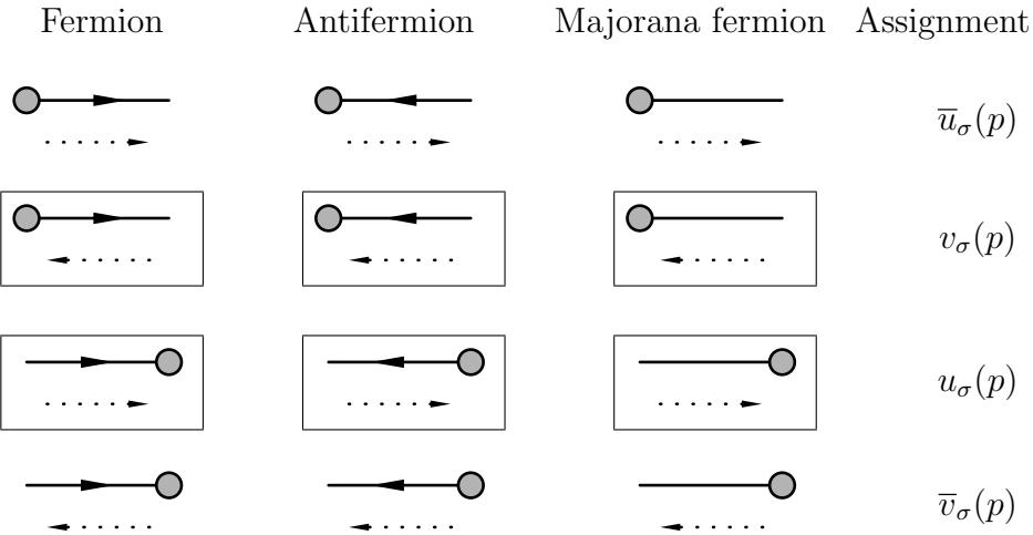
Figure 1: Feynman rules for external fermions for theories with fermion-number violating vertices. Evaluation directions are denoted by dotted arrows. The time flow is from left to right. According to the implementation in O’Mega using an inward pointing evaluation direction only the rules inside the boxes are used.
